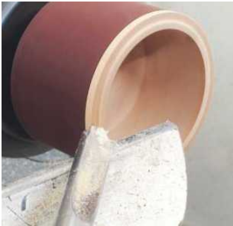
STEP 22. The amount of rim that you leave on is up to you – I think that less is more so I removed some of the apple off the top by using a push cut with a gouge. Make every cut count: a dig in here could destroy all your hard work
